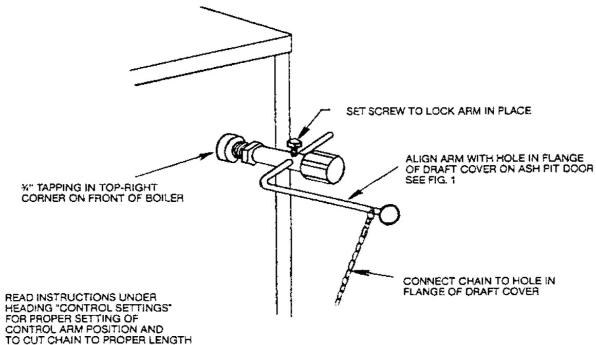
**FIG. 10 DRAFT CONTROL MOUNTING**
