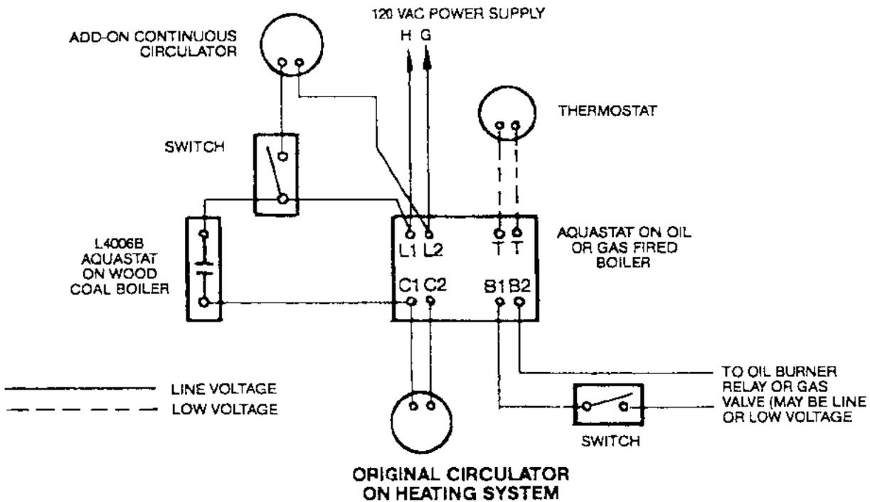
**FIG. 6 WIRING DIAGRAM**
