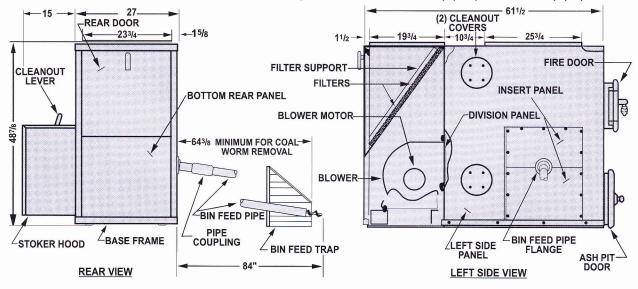
NOTE: Bare heat exchanger dimensions: Width - 301/4", Length - 41", Height - 46"
